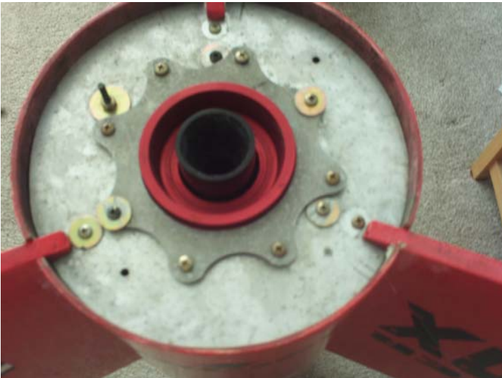
A close up of the installed motor. Its not going anywhere!
